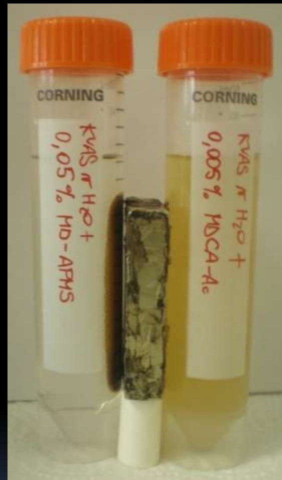
Separation at application of different nanoparticles MD-Si-APMS left ; MD-CA right
